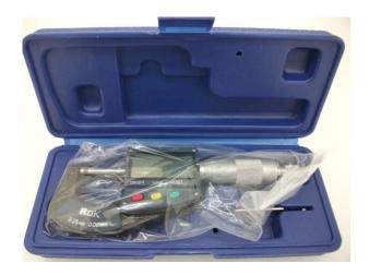
Larger LCD display inch/metric conversion RESET: origin resetting TOL: tolerance setting HOLD: data hold
