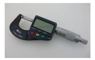
Larger LCD display inch/metric conversion RESET: origin resetting TOL: tolerance setting HOLD: data hold R/A: relative/absolute measurement conversion +:positive setting -: negative setting Range Resolution Accuracy 100-125mm/4"-5" 0.001mm/0.00005" 0.004mm/0.0002
